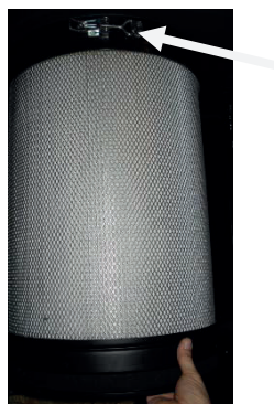
Figure 44: Hold canister from bottom when releasing clamp (top)
