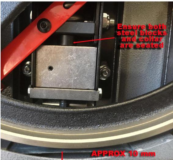
how it should look. (You may initially need to manually pull the top wheel down to achieve this as this is a brand new machine built to exact tolerances) Please ensure you turn the hand wheel the correct way to lower the top wheel and also back off all the ceramic guides to allow the blade to initially run free.
