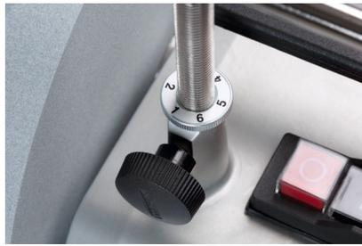
On the new T-8 model, Tormek has integrated the previous mounted sleeves for the Universal Support into the fully cast housing. That guarantees minimal play for the Universal Support; an innovation which improves the control of the sharpening and increases the accuracy of the final results.
