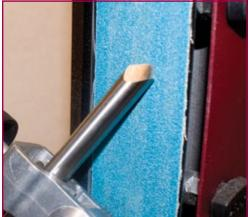
In order to produce a fingernail grind follow the above instruction, the method is the same but with your gouge clamped in the fingernail attachment.
