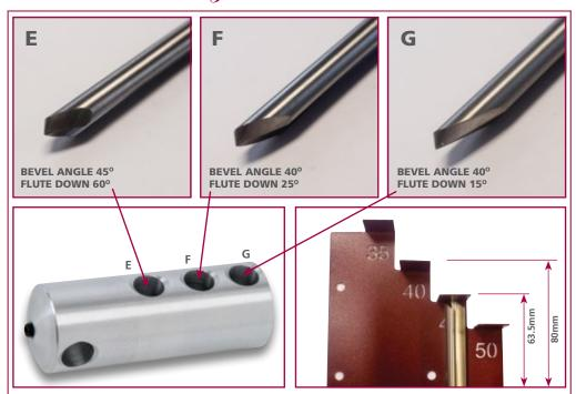
Refer to Step 4 on the previous page to show the grinding method. Please note the fingernail arm and the tool you are grinding should be swung gently from side to side in a flowing motion. Take care not to grind more from the tip than you grind from the sides. You will probably need to spend a little more time on the sides than the tip as there is a much bigger surface area to grind.
